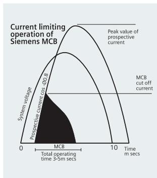
This MCB (16Amps) will allow only 50% of 84,000 ( $A^2S$ ) let-through energy thereby reducing thermal stress to bare minimum value on the downstream equipment.
